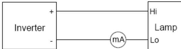
(Figure 1: Measurement of return current)
